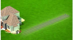
Ground source heat pump coils can be installed vertically or horizontally. Some can also utilize ponds or groundwater.
